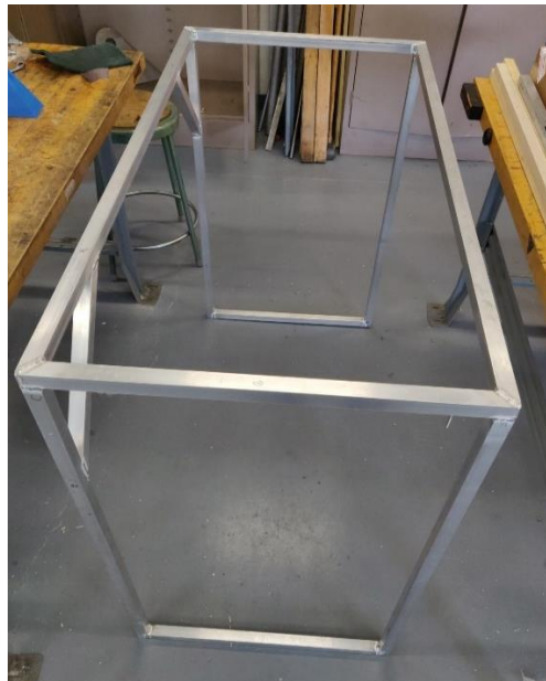
Figure 1. Welded Aluminum Frame for Hood
